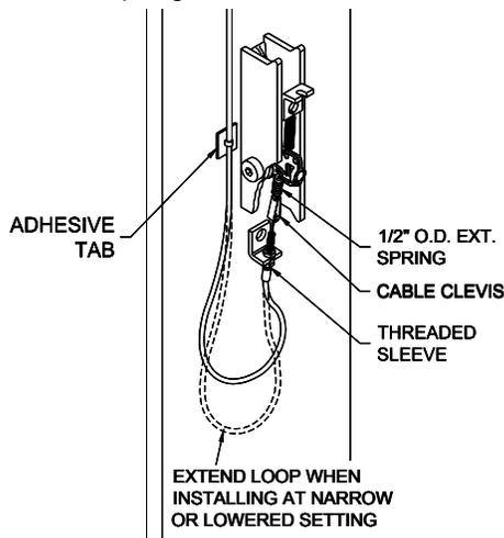
**Fig. 14 – Idler Column Lock Assembly**
