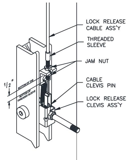
**Fig. 13 – Power Column Lock Assembly**
