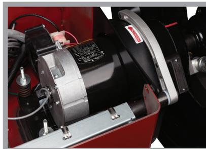
Motor and spindle are combined into a single, pre-balanced assembly that always stays calibrated to zero.
