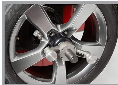
Automatically positions the wheel at the weight placement location and locks the spindle in place for easy, accurate weight application.
