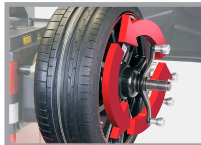
Provides the ability to thread the hub nut at the push of a pedal to improve the ease-of-use and speed of mounting the wheel
