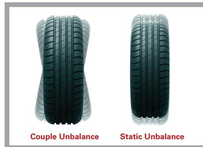
A unique balancing system (unbalance correction methodology) that minimizes both static and couple unbalance
