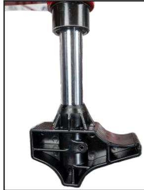
Tool used to push the tire bead into the drop center of the rim, allowing for effortless mounting and dismounting of the tire.
