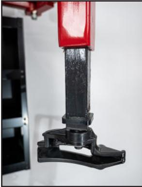
Tool used for mounting and demounting tires without damaging the rim.
